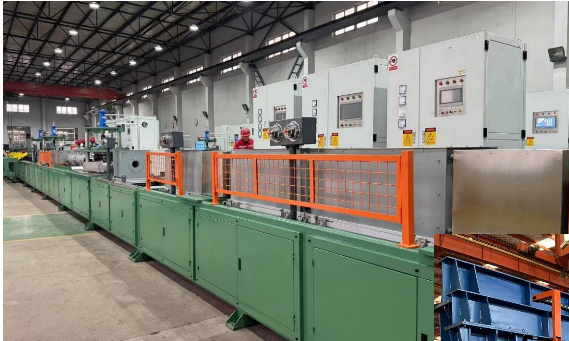
Intermediate frequency heat treatment production line
